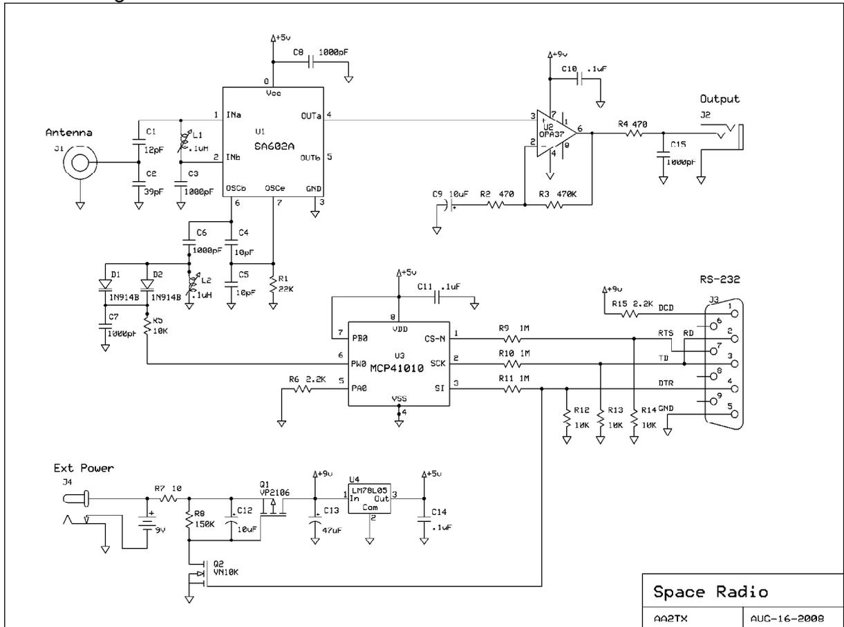
(Figure 2: Space Radio schematic diagram.)
