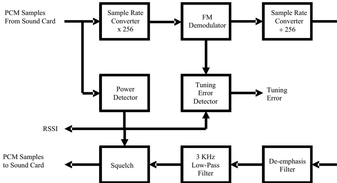
**(Figure 4: Digital signal processing.)**
